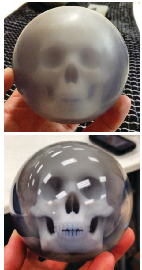
Figure 17: The effect of polishing on transparent and translucent parts.
