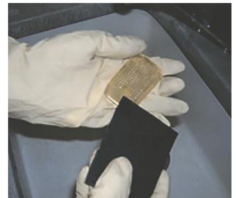
Figure 15: Polishing increases the visual clarity of printed parts.
