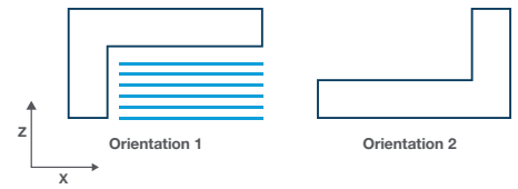
Figure 12: Both options have the same Z height. Orientation 2 will build faster and with less material consumption, and require less post-processing because it does not require support material (shown by the blue lines on Orientation 1).
